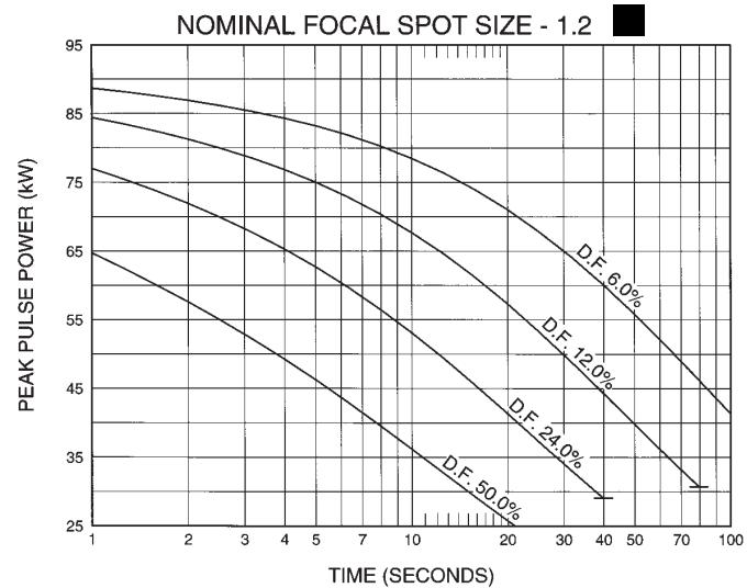
Nominal anode input power for the anode heat content 70%. IEC 60613
