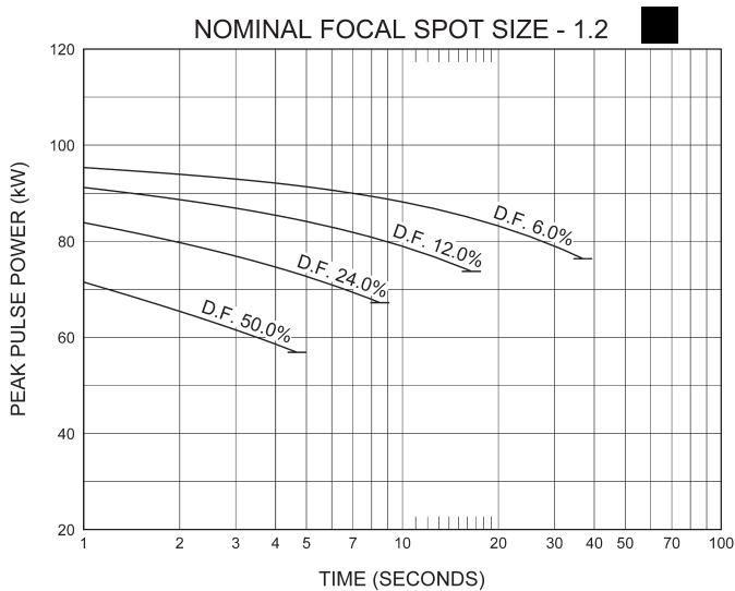
Nominal anode input power for the anode heat content 70%. IEC 60613
