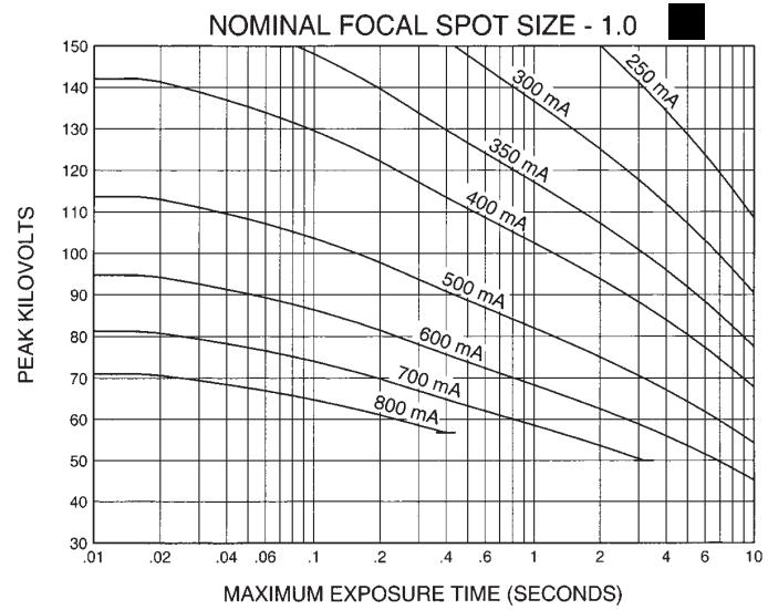
Nominal anode input power for the anode heat content 40%. IEC 60613
