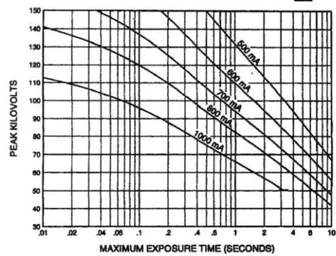
**3 Ø Constant Potential  $\equiv$  50 Hz - 2800 tr/mm**
